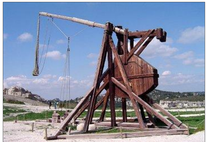
Counterweight trebuchet at Château des Baux, France
