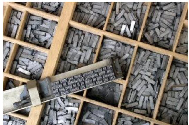
Movable type sorted and loaded in a composing stick.
