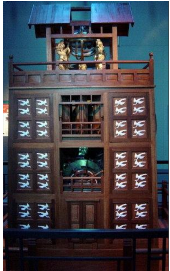
A scale model of Su Song's Astronomical Clock Tower, built in 11th century Kaifeng, China. It was driven by a large waterwheel, chain drive, and escapement mechanism.
