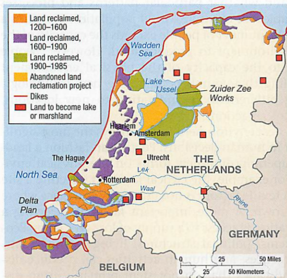
▲ FIGURE 1-44 SUSTAINABLE ECOSYSTEM: THE NETHERLANDS (left) The Dutch people have considerably altered the site of the Netherlands through creation of polders and dikes. (right) A polder in North Holland has been created by pumping the water from the site into the canal.
